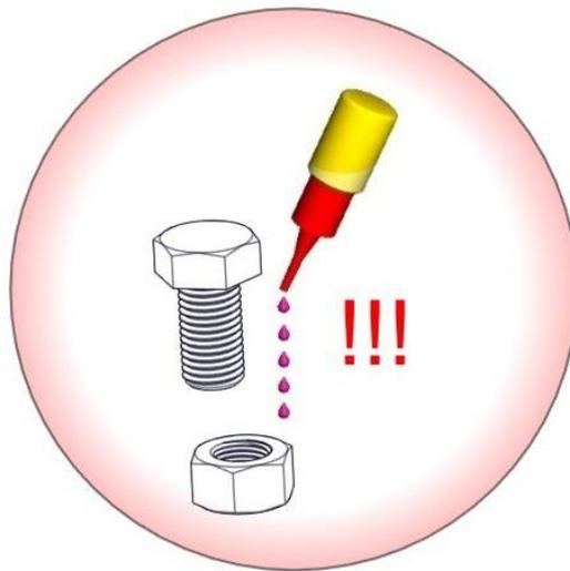
**Glue all screws, nuts and sleeves with loctite.
