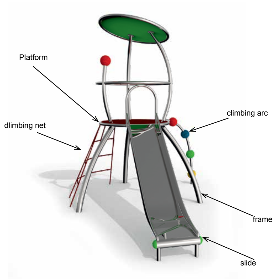
Diagram 1: Overall view of play equipment with description of individual elements
