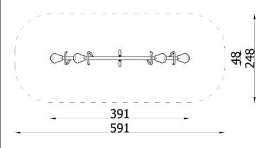
The device is located 60 cm below the ground level. The main swing beam made of steel profile 90 x 90 mm. Handrails made of 38 mm round steel pipe. Seats made of high-pressure polyethylene (HDPE). The construction is placed on a supported steel base. Fasteners and plugs resistant to weather conditions. Steel elements protected against corrosion by powder coating.
