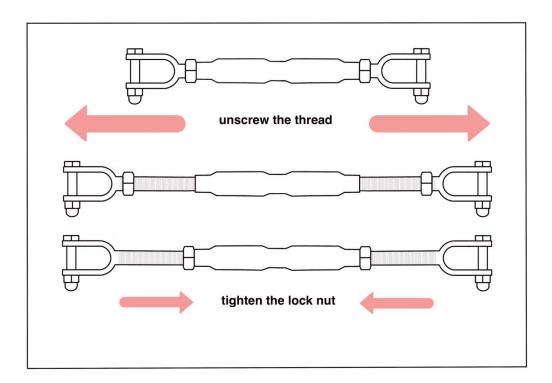
Drawing 5: Functional principle of a turnbuckle
