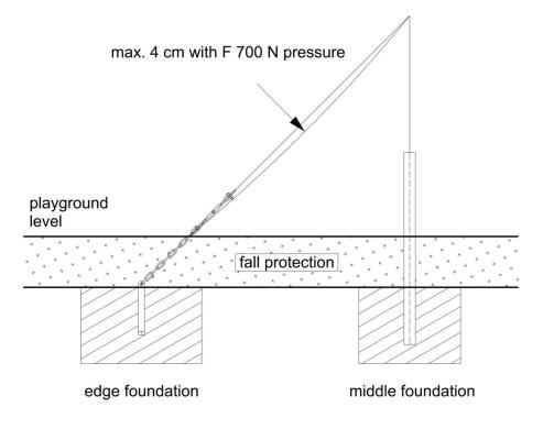
Drawing 6: Pressure-load test
