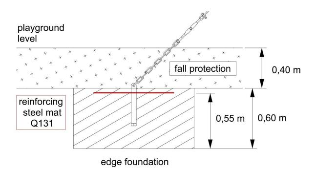
Drawing 2: Construction of the foundation with a reinforcing steel mat
