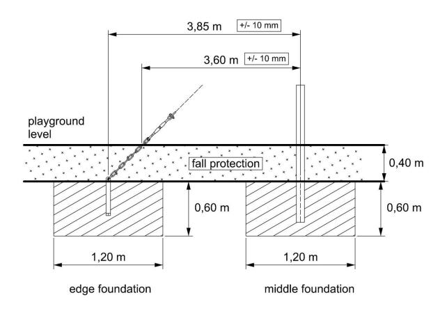
Drawing 3: Distance between the foundations and in the device space
