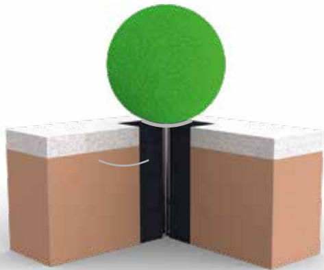
Globes embedded in concrete by means of the floor anchors.
