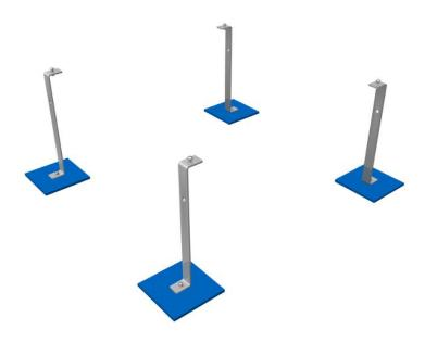
Anchorage component for free standing Park furniture like benches, tables and bicycle racks. Dig about 50 cm deep hole and put the anchor plate to bottom. Screw the metal frame to the plate and other end to the furniture leg. Then cover the hole and compress it. The Foundation set includes four anchoring plates and metal frames.
