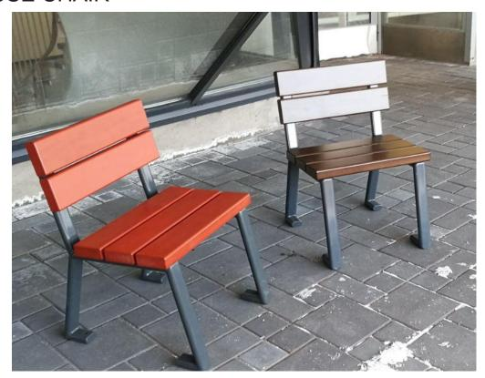
Stable and straight chair for hard use in parks, yards and streets. House is a one seat free standing chair with folded frame paws against ground keeping the bench steady also on grass and sand. For deep mounting on soft soil please use anchor set no 708106 and on hard ground fix with standard concrete screws. Frame material is painted steel, standard colour grey RAL7024, Seat and back rest is painted pine wood, standard colour grey.
