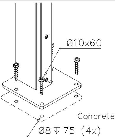
If the product is not installed on one large concrete platform, Option 1.
