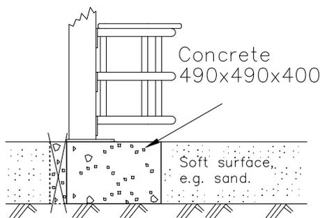
If the product is not installed on one large concrete platform, Option 2.
