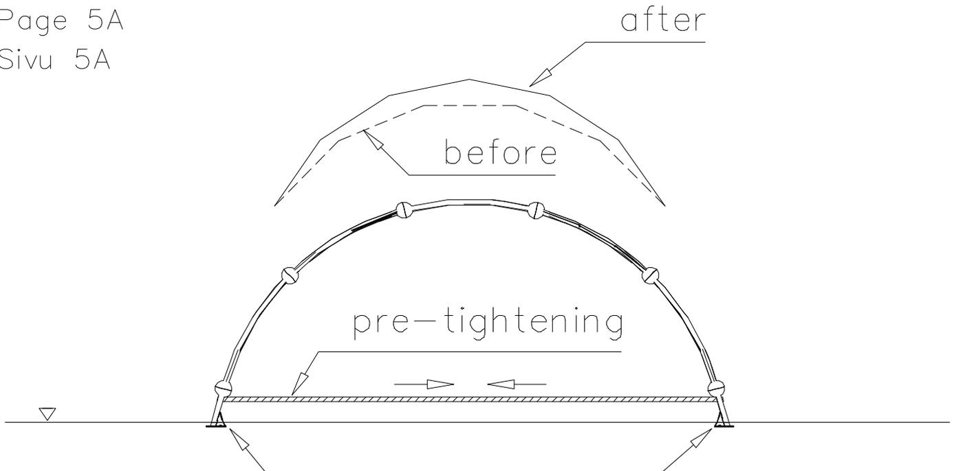
Before the concrete is poured, pre-tension the cage so that the shape of the product is round and even. The tensioning can be done using i.e. chain hoist or lashing straps. Remove the tensioners when concrete has dried enough to prevent the foot from moving.
