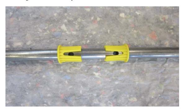
2. Lay the tube with bushings on bottom half of spherical connector. Minimize the gap between bushing sleeve and spherical connector.
