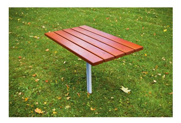
The table is part of Lappset's Scandinavia range, which includes benches with or without backrests. The table has a central leg, which makes it easily accessible for everyone. The Scandinavia range of park furniture is made from pine, has a steel frame, and must be fixed in poured foundations.
