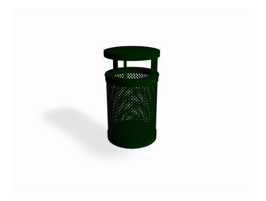
Litter-free playgrounds with Jakob. Jakob is a 35-litre litter bin. The litter bin has several fixing options - either set in poured foundations with a central post (50 mm) (NF2471), wall-mounted using a bracket for wall mounting, or installed using a bracket on an existing post (105-120 mm) (NF2473). Jakob is made from 3 mm powder-coated steel.
