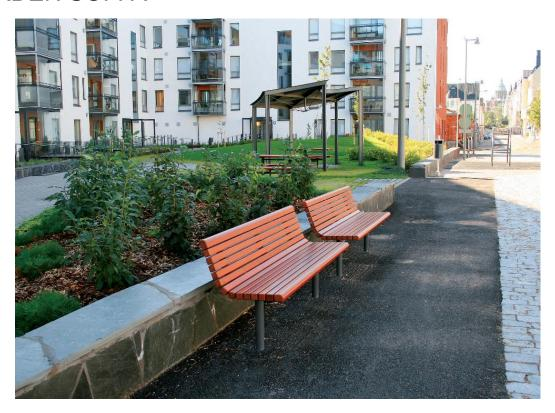
Yarden is a timeless and functional park bench without armrests. The bench seat and back support is made of pine and the frame steel. The bench is also available as free standing (NFJ2012). Yarden park range is available either as free-standing versions or as versions designed for poured foundations. The range also includes a bench without back support, a table and a chair.
