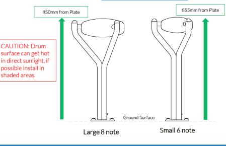
Weight of heaviest part 17.5kg (Large Babel Drum) Weight of heaviest part 13.4kg (Small Babel Drum)
