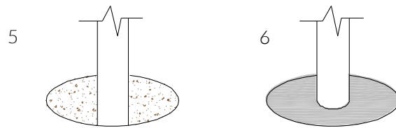
5 Compact base of hole with 50mm of aggregate. Lower ground Fix post attached to instrument into hole (check instrument straight and level before filling with concrete)
