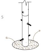
Excavate 1 hole with a 250mm diameter tapering down to 350mm diameter and 650mm depth
