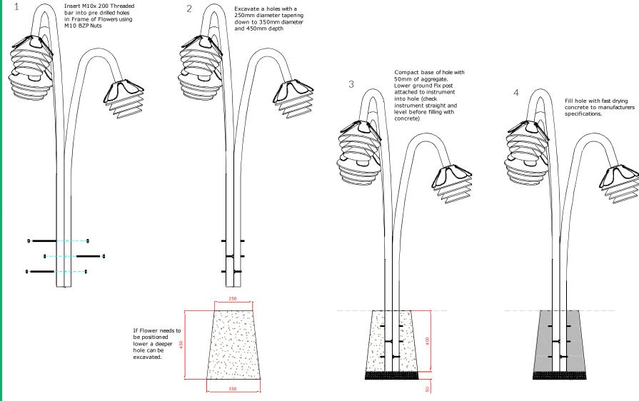
Foundations should not present a hazard. These foundations are recommended as a guide, for more information on foundation details for various surface see Part 1 of BS EN 1176.
